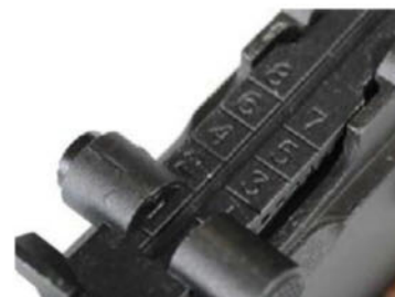
The rear sight of the weapon is a simple iron notched tangent, which can be adjusted from 100 to 800 metres
